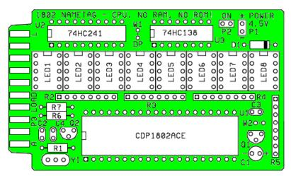
The **LEDs** must be installed with the decimal point in the lower right corner (with the board positioned as shown below). The labeling will be on the right side of the LEDs!
