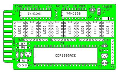
**ICs (Integrated Circuits)** look like black "caterpillars". Bend the pins inward slightly, and insert it onto the board. ICs must face the right way! The end with the notch must match the notch on the board. The text on the IC should be right side up and match the rest of the text on the board. I didn't provide IC sockets, but you can add them if desired.
