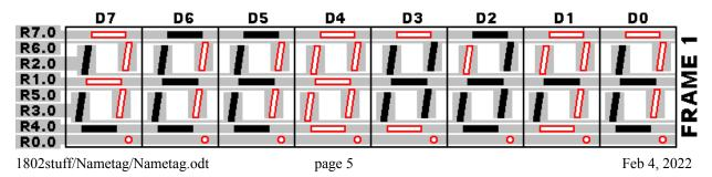
See the long thin gray box on top? It says the top 8 horizontal segments (bits D7 to D0) are to be stored in R7.0 (the low byte of Register 7). Off is "0", and On (filled in) is "1". So R7.0 needs to be programmed with 0110 0100 binary, which is equal to 64 hexadecimal (or 64 hex for short).
