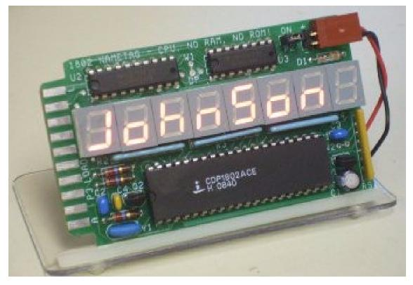
This mad little project is an 1802 Name Tag. It shows how much you can do with an 1802 and an absolute minimum of resources! It's the size of a credit card, and draws about 10ma -- low enough to run for many days on AAA cells or a single 3.6v lithium cell.
